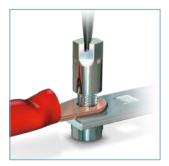
Connection principle of a bolt terminal block
