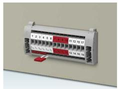
Automatic, leading transformer short circuit implemented with standard plug-in bridges in the plug-in test socket. The positioning of the short-circuit bridges on the outside of the control cabinet is clearly visible.
