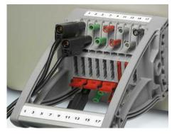
Thanks to the optional use of jumpers, all test circuits can be implemented in the plug. Staggered test sockets enable the use of safety test leads in a confined space.
