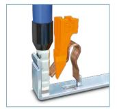
Clamping principle of a push-in terminal block
